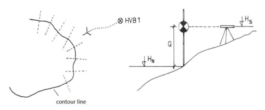
A levelling line starts at the height point HVB1. The line is measured to a point where the horizon of the instruments  $H_S$  is from 1 to 2 m higher than the planned contour line height  $H_N$ .
