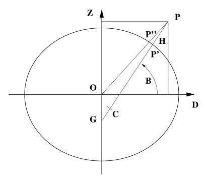
The centre of curvature C of the spheroid corresponding to P' is the point
