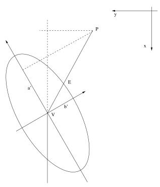
Position of approximate coordinates of an adjusted point with respect to its confidence ellipse is described by two points P and V where point P depicts approximate coordinates and V adjusted coordinates. Point E is the intersection of oriented half-line VP and the confidence ellipse. Coefficient g is defined as the ration of abscissae
