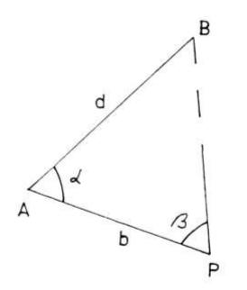
The horizontal angles  $\alpha$  and  $\beta$ are measured at the points A and P, the horizontal distance b is measured by a tape:
