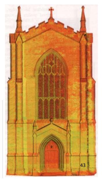
3D model, replacing of the point cloud by geometric primitives
