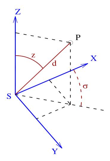
Measured: slope distance *d* horizontal angle *ω* zenith angle *z*
