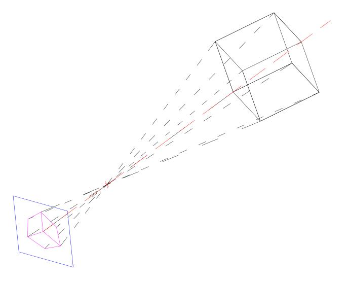
These parameters must be known for determination of a shape, size and spatial position of an object :
