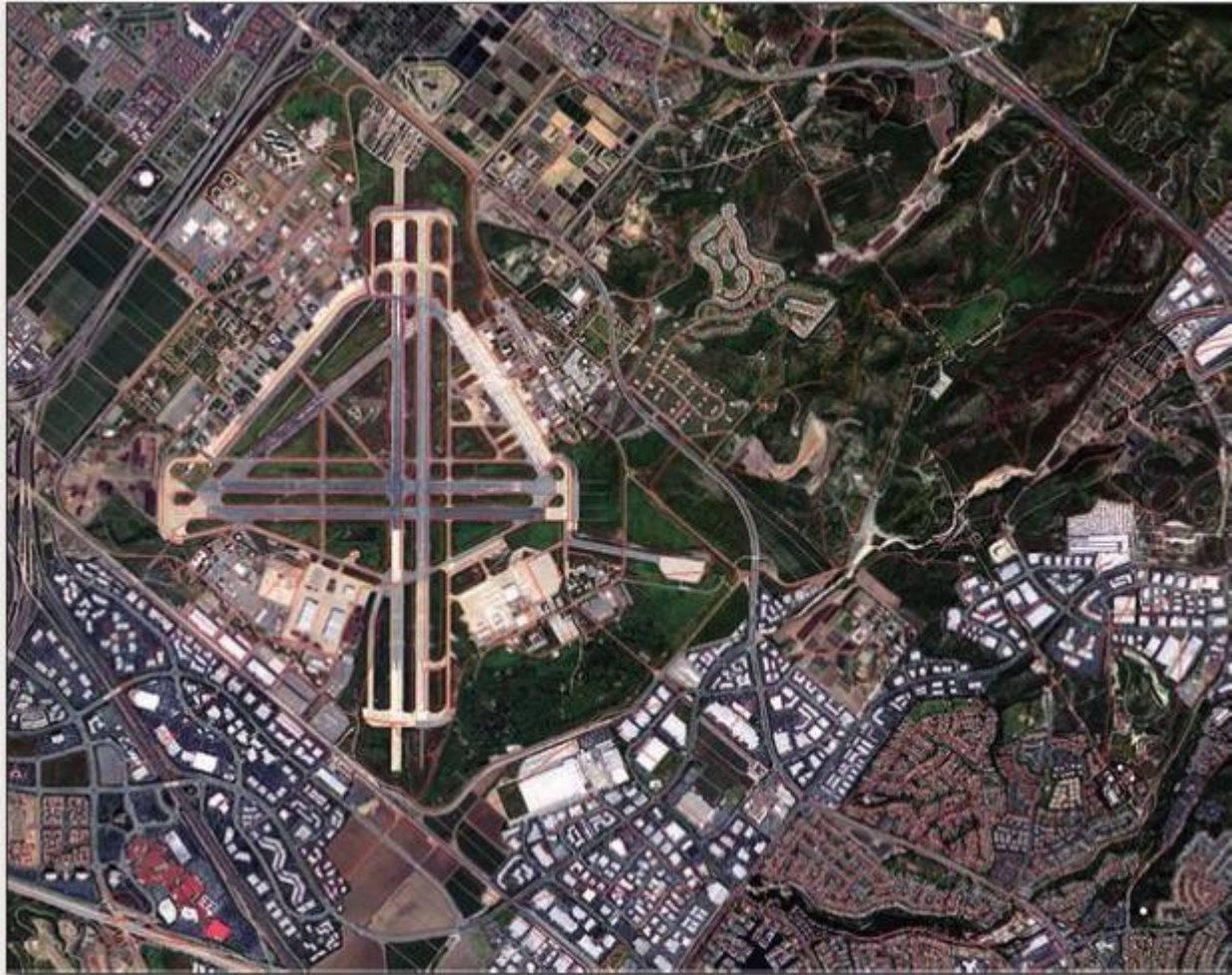
Figure 2: Full resolution orthorectified RapidEye image of Irvine corrected without GCPs overlaid with USGS 1:24000 vectors
